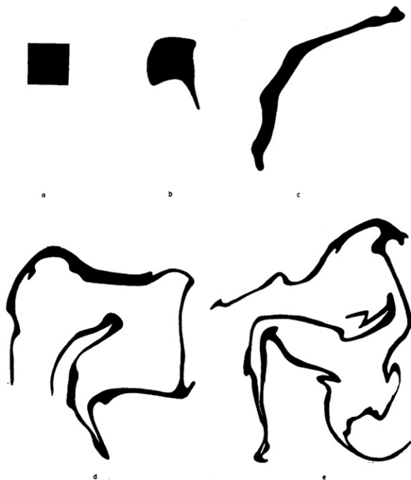
FIG. 7-14. Sketch (Welander 1955) showing the effects of “stirring” of a two-dimensional flow on small regions of dyed fluid. Dye is carried into long streaks of greatly extended boundaries where very small scale (molecular) mixing processes can dominate. (© 1955 Pierre Welander, published by Taylor and Francis Group; https://creativecommons.org/licenses/by/4.0/ .)
